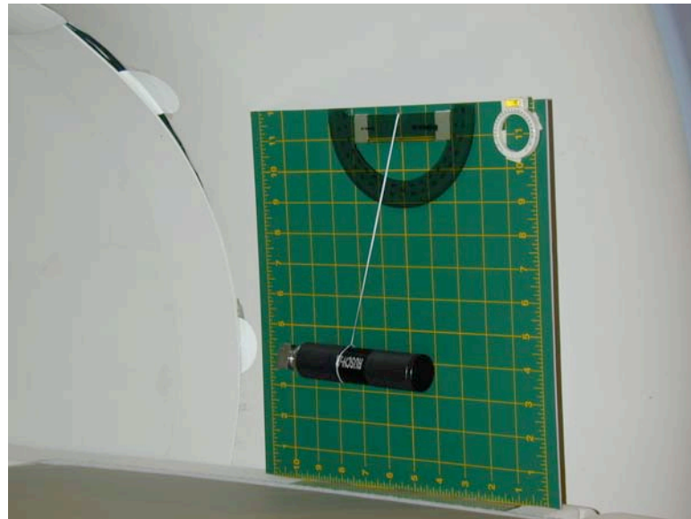
FIGURE 3a. The deflection angle test conducted at 3-Tesla on Rusch Laryngoscope handle with battery. Note the deflection angle of 14-degrees measured in the 3-Tesla MR system.
