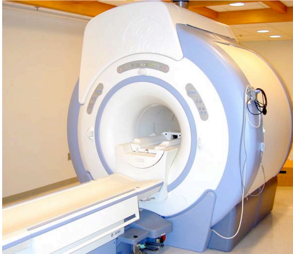
FIGURE 2. The 3-Tesla MR system (General Electric Healthcare, Milwaukee, WI) used for MRI testing.
